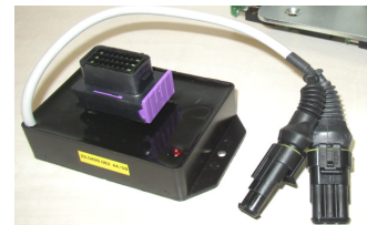
Lift & Lower Electronic Control and PWM driver
