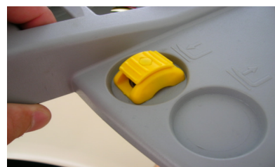
Proportional Roller Switch for Manual Lift & Lower Control
